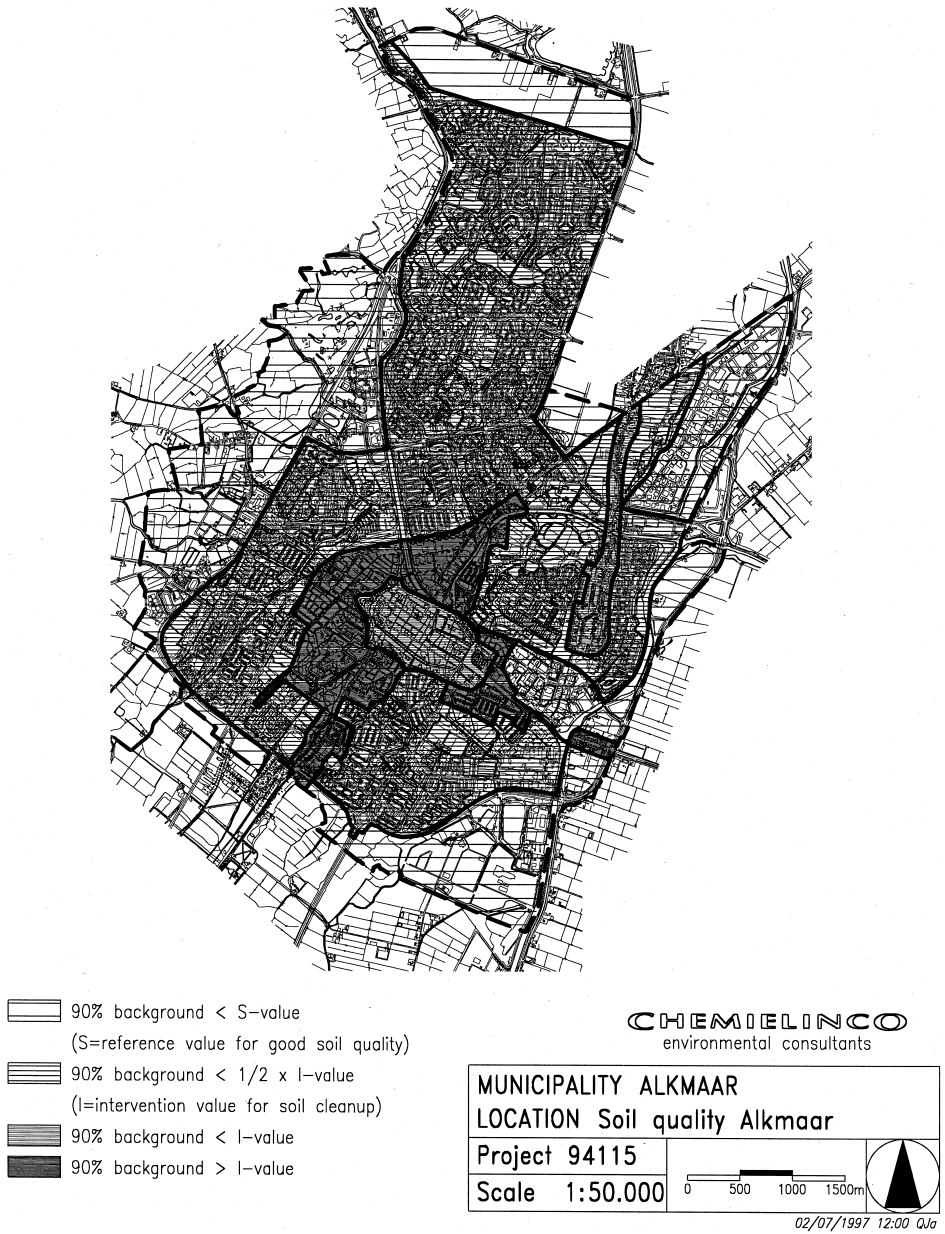
Fig. 1. Map of background values of soil contaminants in the city of Alkmaar.
